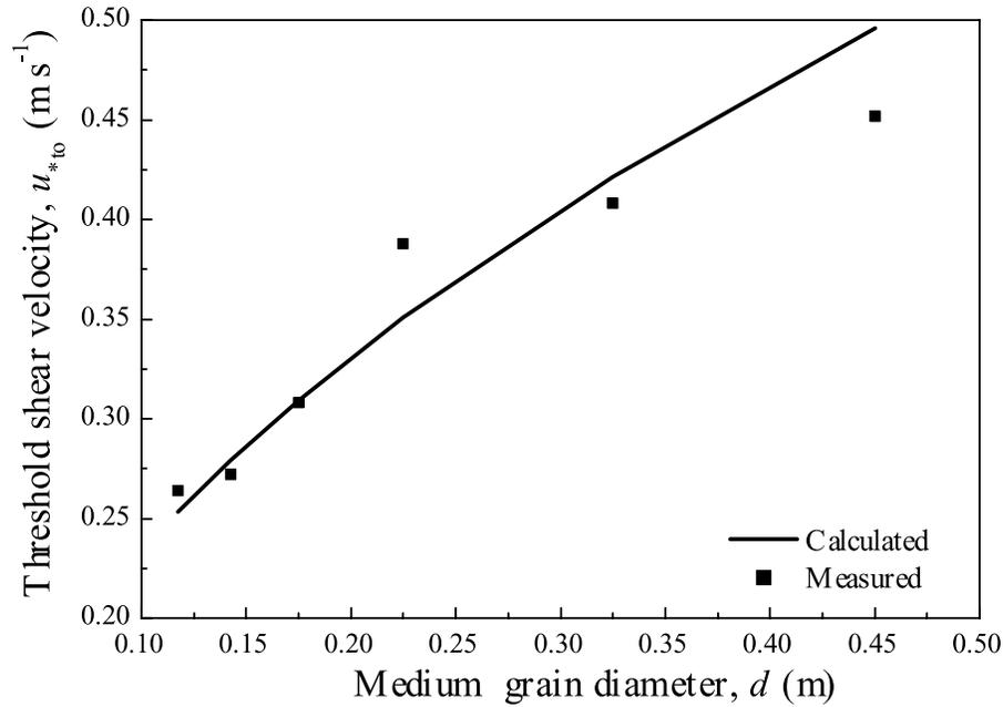
**Figure 3.** Threshold shear velocity of dry sand ( $u_{*to}$ ) versus particle size ( $d$ ). Wind tunnel results are compared against the model derived in this study.
