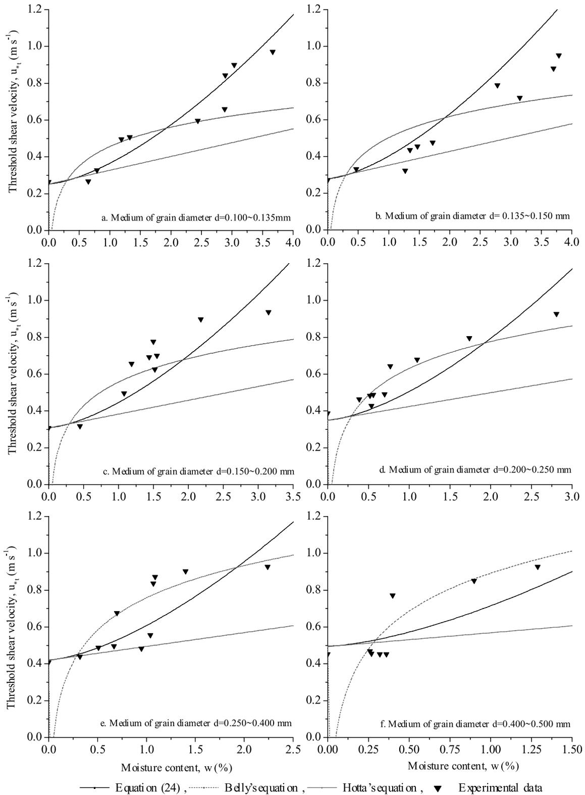
**Figure 5.** Comparison of the threshold shear velocities predicted by Belly's, Hotta et al.'s and our formula with the threshold shear velocities obtained in experiments for six size samples: (a) 0.100–0.135 mm, (b) 0.135–0.150 mm, (c) 0.150–0.200 mm, (d) 0.200–0.250 mm, (e) 0.250–0.400 mm, and (f) 0.400–0.500 mm.
