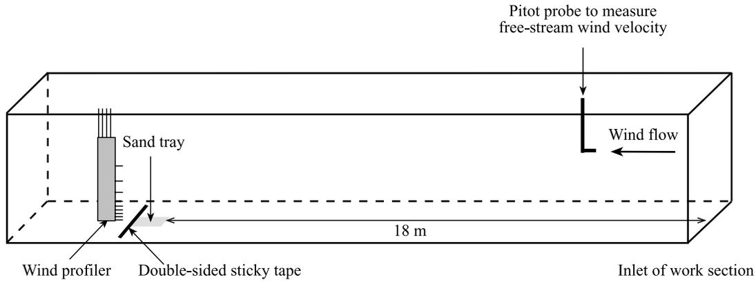
Figure 2. Layout for the experiments.
