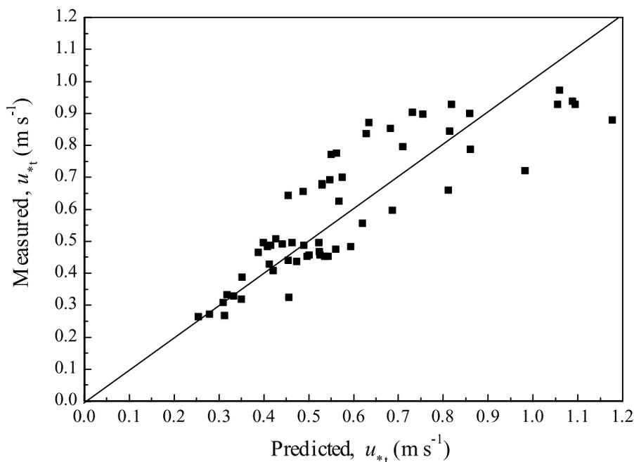
**Figure 4.** Comparison of the measured threshold shear velocity with the threshold shear velocities predicted using equation (26).
