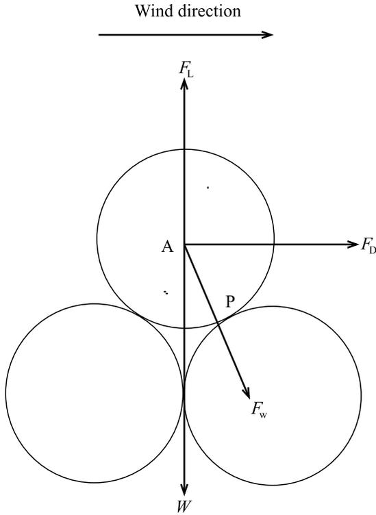
**Figure 1.** Sketch of the forces on a particle at the initiation threshold.
